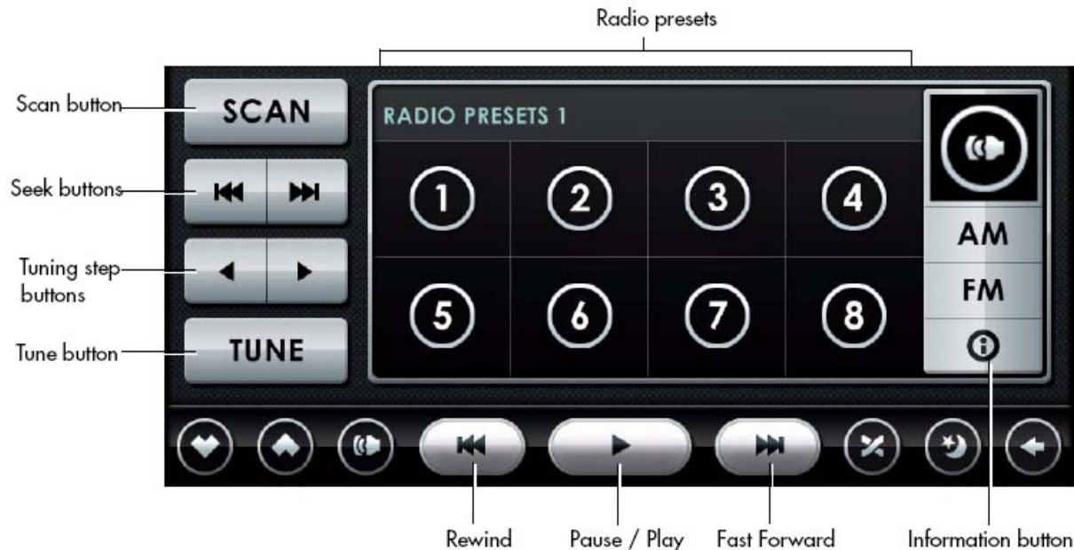
Figure 4-7: FM/AM Radio controls
